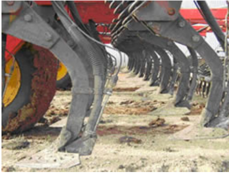
Fertiliser injection set-up at each tine
