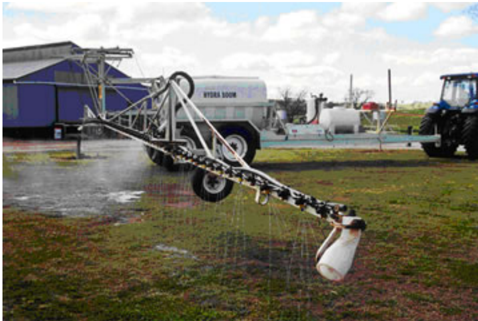
Wayne's Hydra boom displaying dribble jets as opposed to fan jets (middle of boom)
