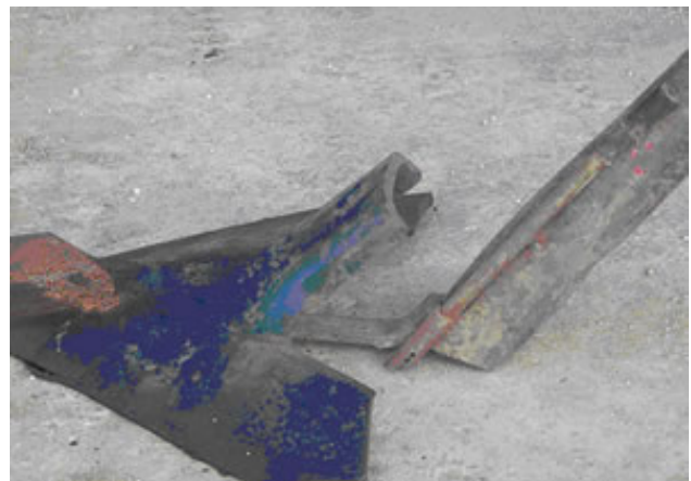
Injector tube directs fluids ahead of the seed
